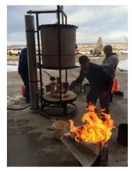
Ceramic pieces are placed in the Raku kiln and in about an hour the pieces have reached a temperature of 1800° fahrenheit. The top of the kiln is lifted and the glowing red-hot pieces are removed from the kiln using tongs and placed in cans full of combustible materials.
